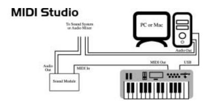
In this scenario, it may not be necessary to apply external power to the Oxygen 8. With the power switch set to "Power Off," the Oxygen 8 receives power from the USB port on your computer. It is recommended that you either plug directly into the USB port on the computer, or use a powered USB hub. You may also choose to use power from batteries or an external power supply.
